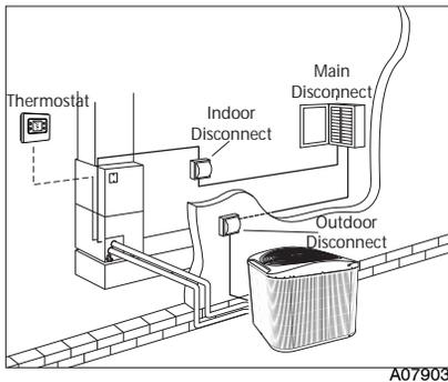
Fig. 1 - Electrical Disconnects
