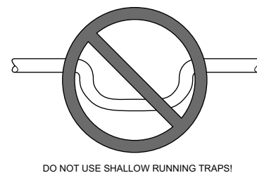
Fig. 12 – Insufficient Condensate Trap
