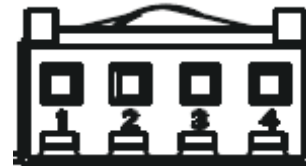
Fig. 7 – Sensor Wire Harness Pin Layout
