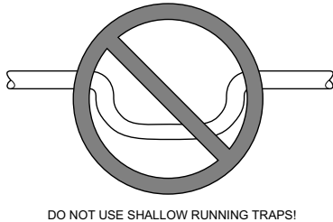
Fig. 5 – Insufficient Condensate Trap
