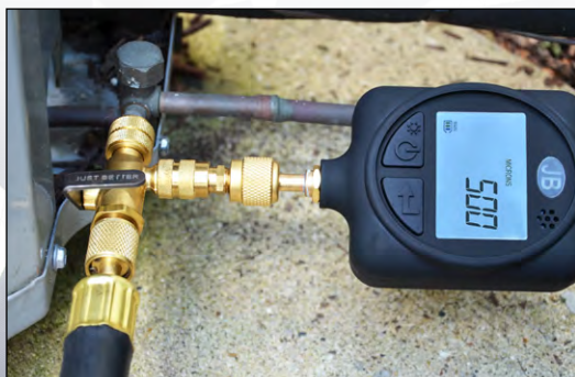
Easily attach and protect vacuum gauge with the slide valve side port
