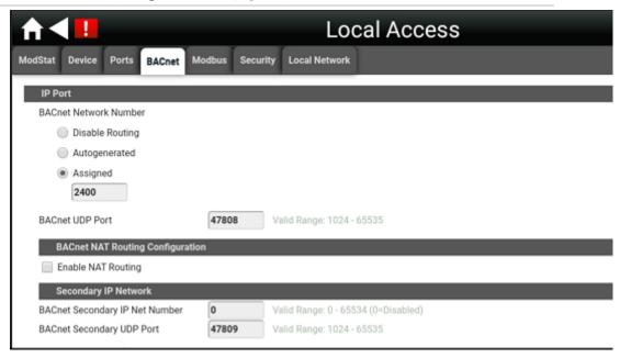
Local access browser for IP-based controllers. View and configure controller information using the tabs at the top of this screen.
