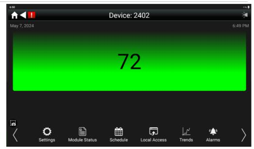
Displays the BACnet device instance number, the controller's date and time, temperature read from the controller's prime variable, and zone color. Touch a button to jump to the **Settings**,
