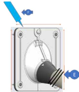
7. Use the zip ties to tie the flexible sleeve around the lineset bundle, as shown in **E**
