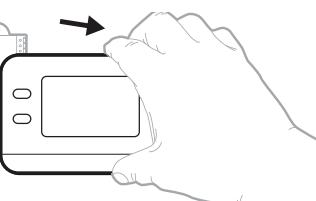
Insert AA batteries for primary or backup power
