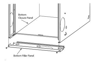
Fig. 4 – Removing Bottom Closure Panel for Non-Condensing Furnaces
