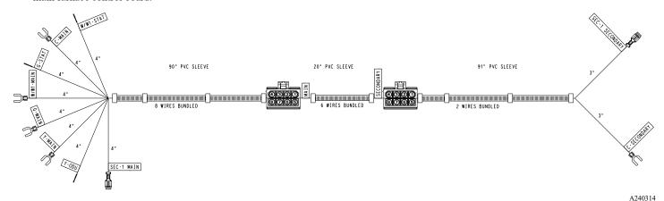
Fig. 21 – Power Wiring Harness (A2L Leak Dissipation)
