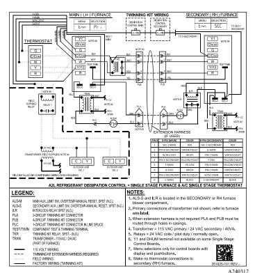
Fig. 22 – A2L Single Stage Wiring Diagram
