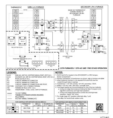
Fig. 26 – Two-Stage Furnace
