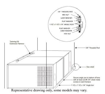
Fig. 13 – Suspended Back-to-Back for Non-Condensing Furnaces ONLY.
