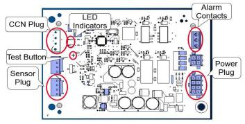
Fig. 20 - Leak Dissipation Control Board
