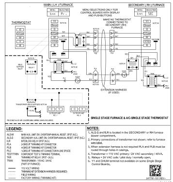
Fig. 24 – Single-Stage Furnace with Single-Stage Thermostat
