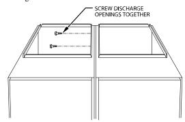
Fig. 7 – Furnaces Together at Discharge Opening
