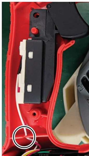
2) Press the Switch Wire into the groove of the Handle Support.
