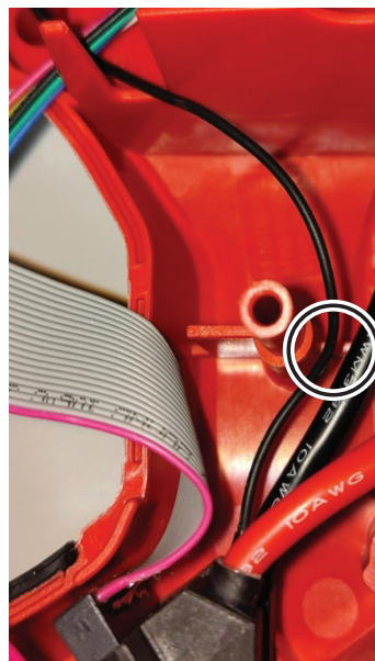
3) Press the thin black Ground Wire into the groove of the Handle Support.
