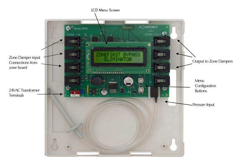
The Bypass Eliminator<sup>™</sup> (Model BPE) Control is an interface between a ZONEFIRST Zone Control Panel and its zone dampers. The BPE is used to eliminate the need for a traditional separate by-pass duct and damper directed back into the return duct. The BPE can **ONLY** be used with ZONEFIRST'S Plug-In Zone Dampers and control panels.
