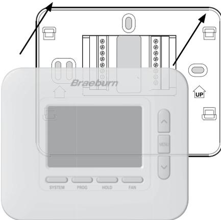
**Once you complete the wiring in Section 3, attach thermostat to sub-base and then configure the Installer Settings in Section 5.**
