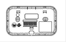
If new mounting holes are needed, mark the placement of the new mounting holes through the thermostat base. Using a 3/16" drill bit, drill the holes you have marked and insert the supplied wall anchors.
