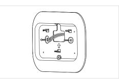
Feed the wires through the hole in the trim plate and screw the trim plate to the wall
