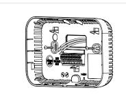
Feed the wires through the hole in the back housing of the thermostat and then screw the back housing to the wall
