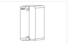
Insert mounting screw into top of junction box until there is approximately 1/8" gap between the screw head and the wall
