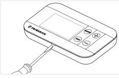
Use a flat head screw driver to separate the front and back housing of the thermostat
