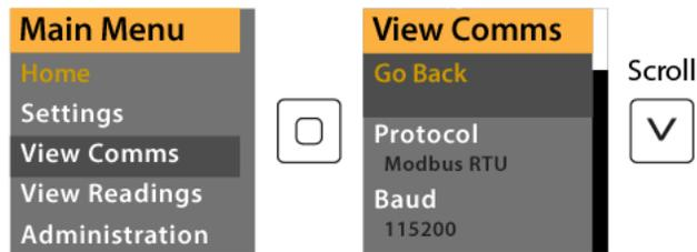
To view current readings without configuring display, navigate to “view readings” in the main menu.
