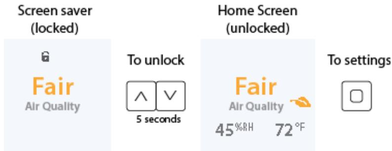
To change any setting, press enter to see setup menu and navigate to desired parameter and press enter again to choose. For example, to adjust display parameters, access the setup menu by pressing the 'enter' button once to access the setup and once more to access the "display" menu and then select "center display".
