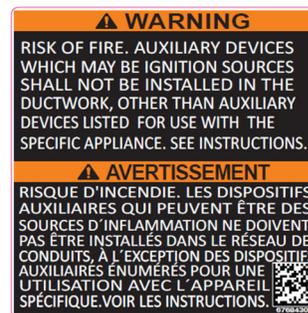
3. Apply remaining labels to the outside of the unit, upright in a location that is visible to service personnel and future inspectors.
