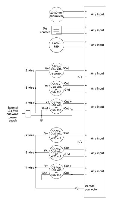
**NOTE** For a loop-powered 4-20 mA sensor, wire the sensor's positive terminal to the **+** terminal on the TV-UCXPI048's **24 Vdc** connector. Wire the sensor's negative terminal to an input's **+** terminal.
