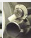
LOCK TUBES USING RETENTION CLIP
