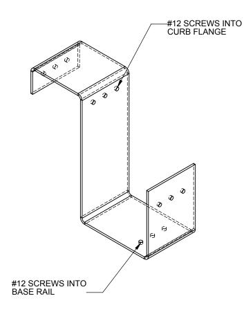
Notes: 1. MATERIAL: 14 ga. GALVANIZED STEEL CURB SHOWN IS CDI STANDARD CONFIGURATION CDI RESERVES THE RIGHT TO CHANGE LAYOUT WITHOUT NOTIFICATION. IF CURB IS NEEDED IN A DIFFERENT CONFIGURATION CDI MUST BE NOTIFIED PRIOR TO PLACING AN ORDER.
