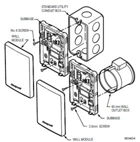
Figure 2. Installing sub-base on the wall
