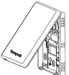
Figure 1. Removing the module from its sub-base
