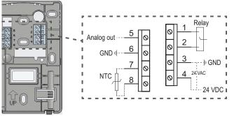
Figure 3. Typical wiring connections
