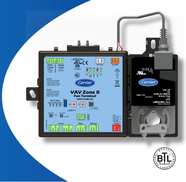
The VAV Zone II Fan Terminal controller provides zone level temperature and air quality control for a variety of pressure-independent VAV applications. This advanced controller features a separable actuator for easy installation onto fan-powered or single-duct air terminals. It also features native BACnet communications and plug-and-play connectivity to the Carrier i-Vu Building Automation System.
