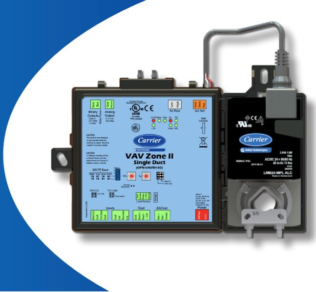
The VAV Zone II Single Duct controller provides zone level temperature and air quality control for a variety of pressure-independent VAV applications. This advanced controller features a separable actuator for easy installation onto single duct air terminals. It also features native BACnet communications and plug-and-play connectivity to the Carrier i-Vu Building Automation System.
