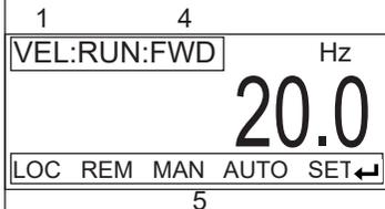
In the Process Control Mode, instead of the Output Frequency, the Process Control Setpoint is displayed.
