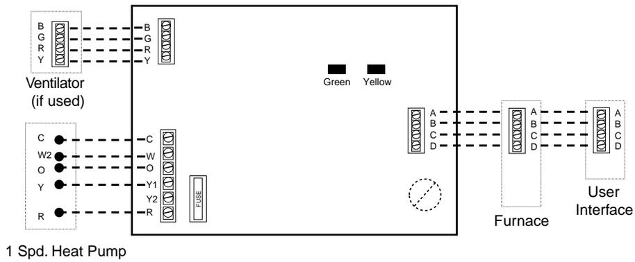
**Fig. 3 — Variable-Speed Furnace with 1-Spd. Heat Pump (Dual Fuel)**
