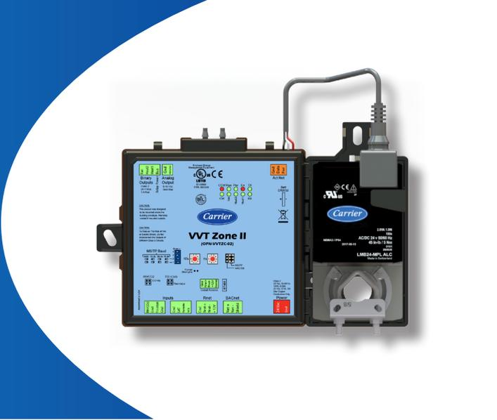
The VVT round zone damper with the VVT Zone controller is a component of Carrier's i-Vu Building Automation System. It provides accurate and precise airflow for VVT applications. The factory-integrated VVT Zone controller maintains space temperature by modulating the proper amount of supply airflow through its damper.
