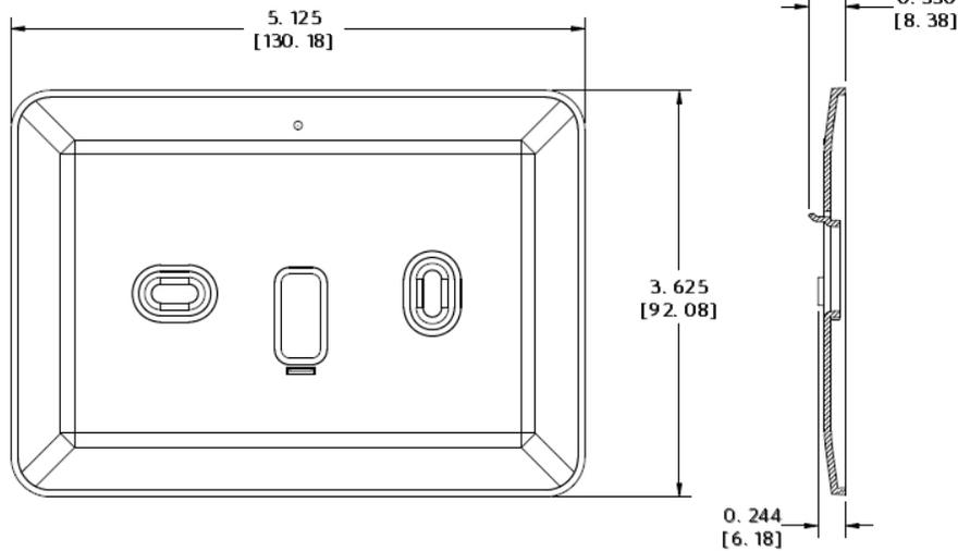
**Fig. 5 – Smart Sensor Trim Plate Dimensions**
