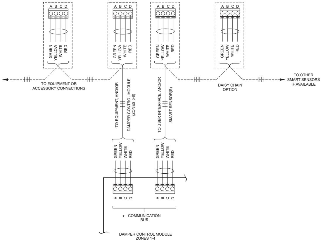
**Fig. 2 – Typical Smart Sensor Wiring Diagram**
