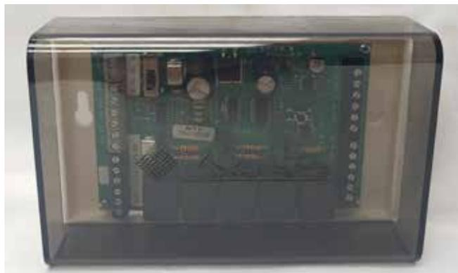
The RLYX is a communicating device equipped with 5 SPST relay terminals switched between a single Common terminal (NOT as dry contacts independent from each other). The RLYX can be used to control loads such as fans, pumps, blowers, lighting, or any load that can be operated using low voltage signals of 24VAC or less. When a relay is energized a circuit is completed between Common and the corresponding relay terminal (i.e. Common and R1, Common and R2 and so on). Status of the relays are
