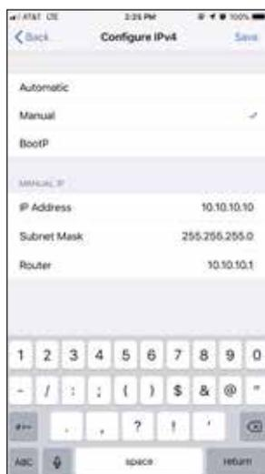
5. Under **IPV4 ADDRESS** tap **Configure IP**. On the next menu tap **Manual**. A menu will appear just below labeled **MANUAL IP**.
