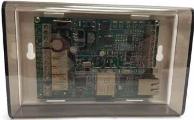
The GEN UC (Part# GENUC) is a microprocessor based, digital communicating controller designed to communicate and control stand alone G/E or HP units, either RTU or split type systems, remotely over the internet. The GEN UC will communicate and control up to 20 SATouchX's. The GEN UC is expandable using up to 20 add-on GEN UC RM controllers that are daisy chained together via the RS-485 communications link, providing system expansion up to 400 units.
