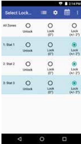
Thermostats can be locked independently or globally through your Mobile device, when a thermostat is locked the end user will have limited operation (+/- 2°) or no variance (0°) of the thermostat from heating or cooling set points.
