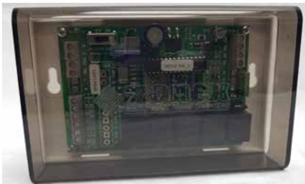
The GEN UC RM is a micro-controller based, auto changeover Universal Gas/Electric or Heat Pump system controller (Part# **GEN UC RM**), designed to work with the GEN UC controller to provide expansion capability to support additional stand alone units. The **GEN UC RM** supports up to 20 SATouchX's. The **GEN UC RM** gathers information every 60 seconds from each thermostat while communicating with the system over a 2-wire data link.
