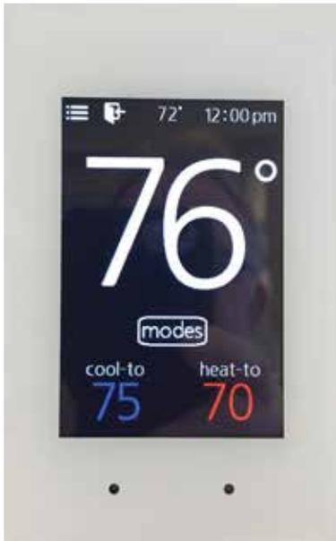
The SATouchX is a universal programmable G/E or H/P thermostat, microprocessor based, auto changeover, stand alone thermostat used to control stand alone units in the GEN UC system. The SATouchX is configured for Gas/Electric (2H, 2C) or Heat Pump (3H, 2C) with selectable fan operation. The SATouchX reports the room humidity, supply and return air temperatures and has a large, easy to read LCD display.
