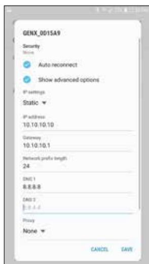
6. Under **"IP settings"** change **"DHCP"** to **"Static"**, under the **IP address** field type in 10.10.10.10, under the **Gateway** field type in 10.10.10.1 under the Subnet field (if present) type in 255.255.255.0 and then save the settings or tap **"Connect"**.
