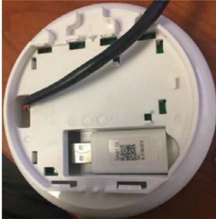
**Fig. 5 — Insert Wi-Fi Dongle on USB Port**
