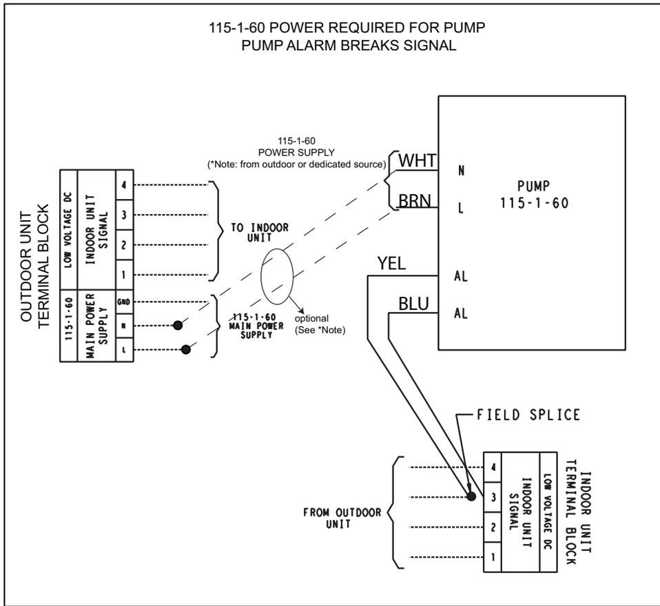
Fig. 8 - (115-1-60) WIRING SCHEMATIC
