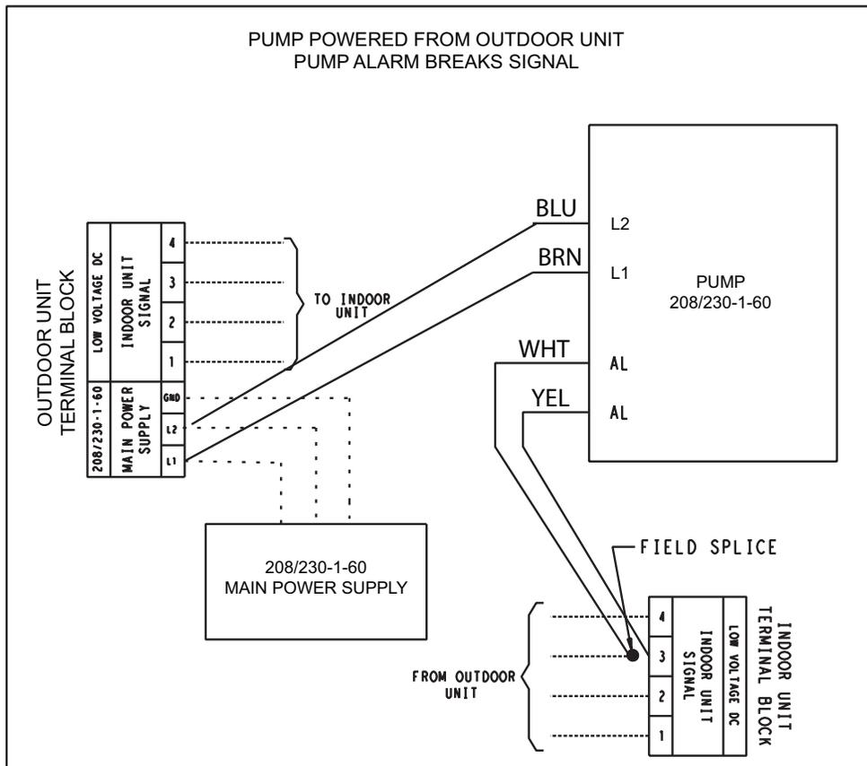
**Fig. 10 - (208/230-1-60) WIRING SCHEMATIC**
