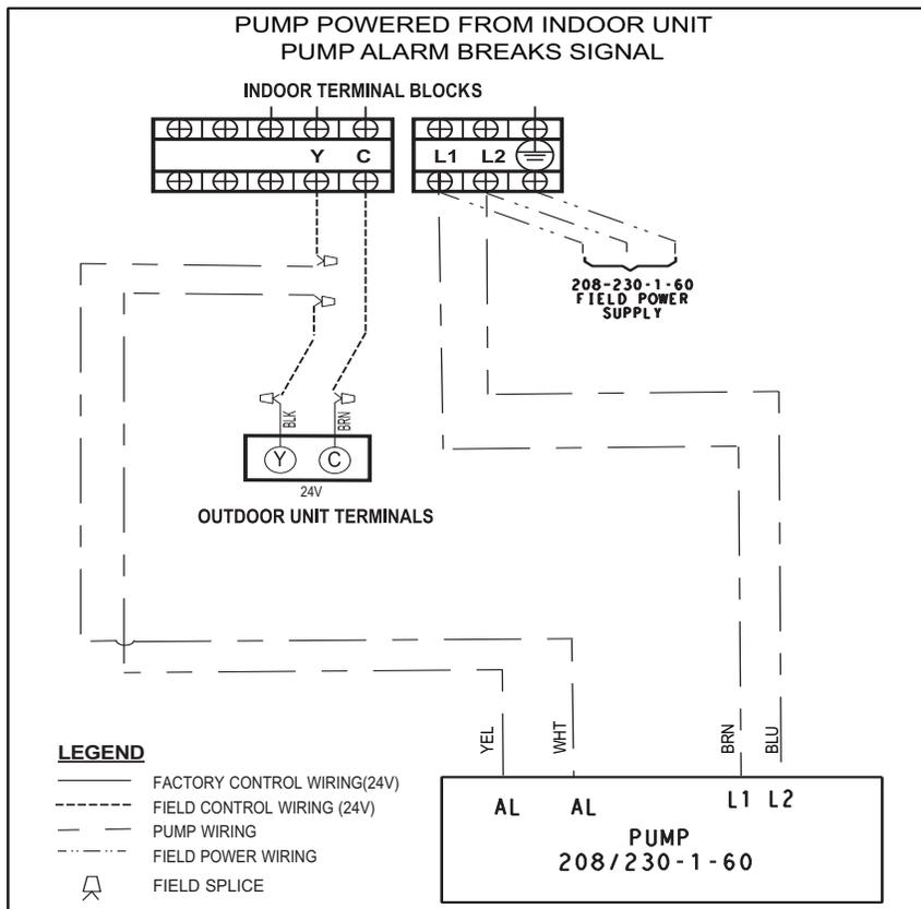
**Fig. 26 – 208/230-1-60 Pump in a 208-230-1-60 40MK\*F Under Ceiling AC Unit - WIRING SCHEMATIC**
