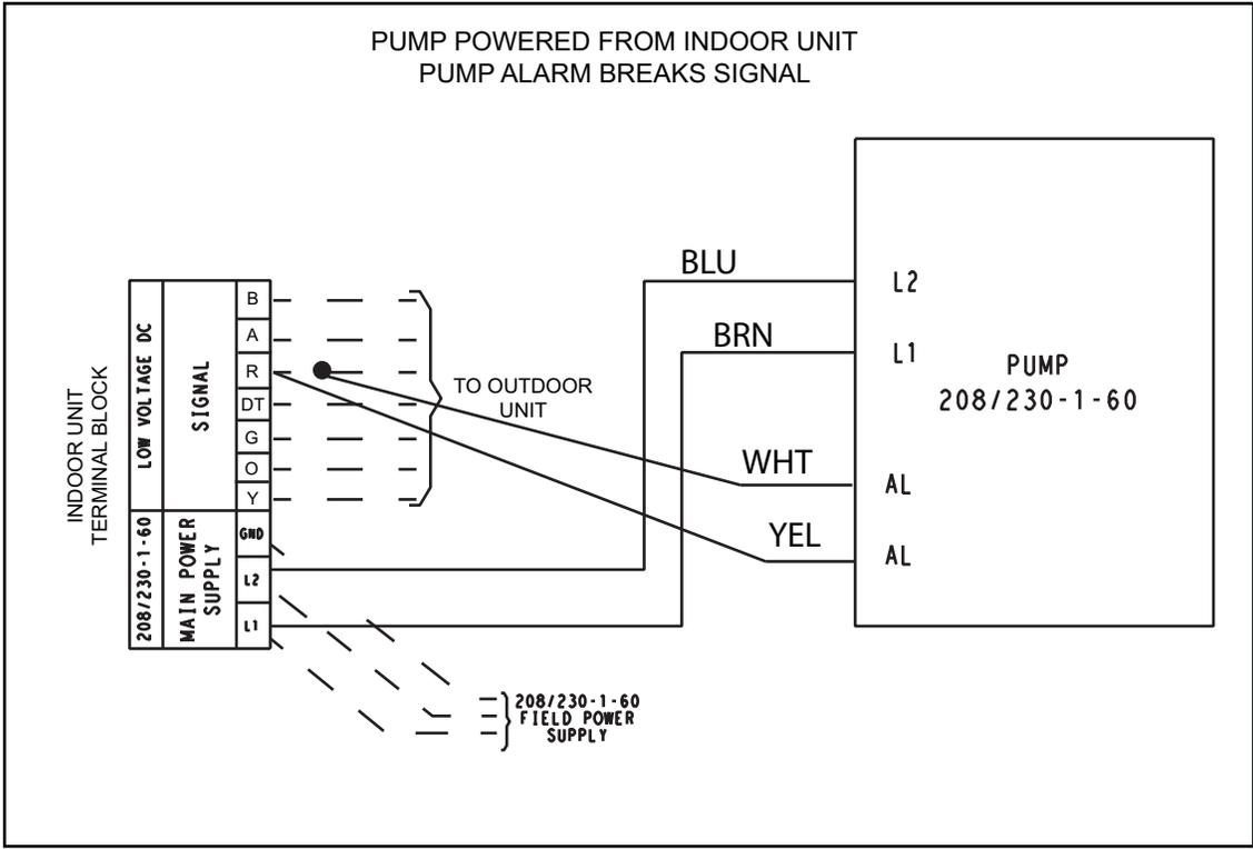
Fig. 12 - (208/230-1-60) WIRING SCHEMATIC
