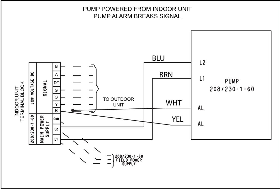
Fig. 13 - (208/230-1-60) WIRING SCHEMATIC
