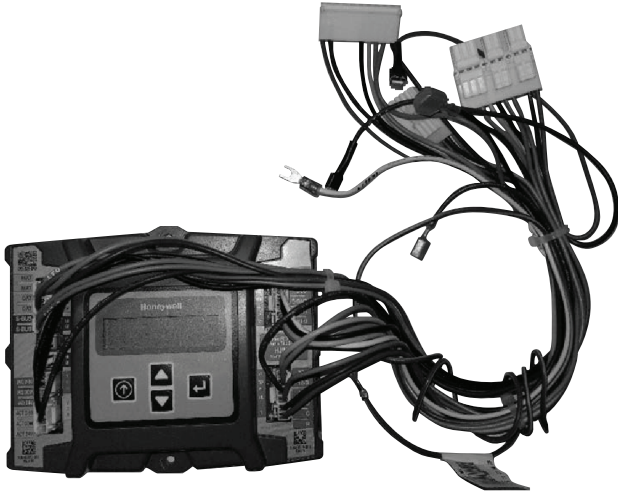
Fig. 26 — Remove Complete Harness Factory-Attached to W7220 Controller
