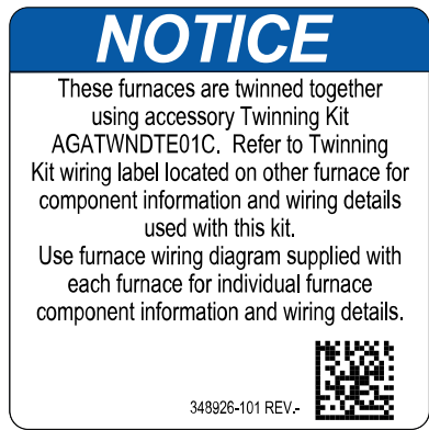
Fig. 23 – Example of Twinning Reference Label
