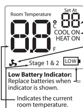
Stage 1 and 2 indicate the stages of HEAT that are active.
