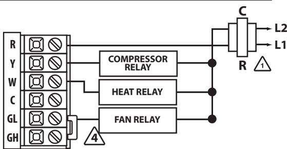
**Typical 1H/1C Heat Pump System: 2 Speed Fan**
