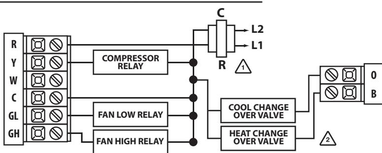
**Typical 2H/1C Heat Pump System: 2 Speed Fan**
