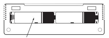
Insert 2 AA Alkaline batteries (included). High quality Alkaline batteries are recommeded.
