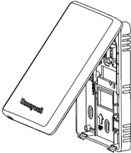
**Figure 1. Removing the module from its sub-base**
