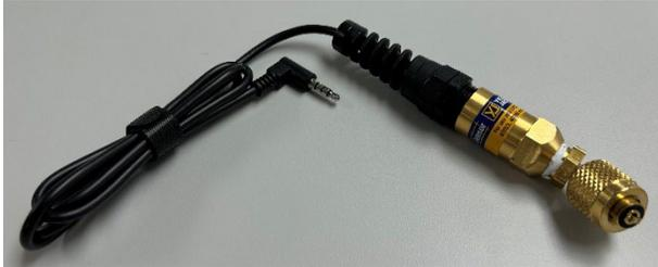
Figure 9: P/N 67044 Vacuum Sensor
