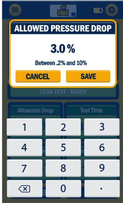
Figure 23: Pressure Decay Test – Set %
