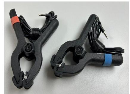
Figure 6: P/N 40846 Included TITAN® Temperature Clamps
