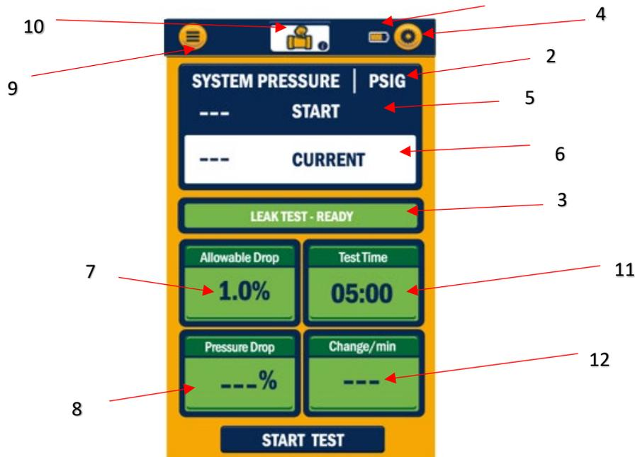
Figure 21: Pressure Hold – Pressure Decay Test Diagram
