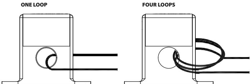
For applications in which the normal operating current is greater than 150 Amps or for conductor diameters larger than 0.530" (1.35 cm) in diameter, an external 5 Amp Current Transformer must be used as shown in **Figure 4** below.
