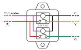
The power for the relay coils travels through the purple and black wires. The load side of the relays is not connected to the coil side.
