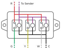
**Note:** Applying 24VAC to the Sender's yellow wire will activate both the green and yellow relays on the Receiver. The Model 3000's yellow, green, and white wires can not used for a common connection 'C'.
