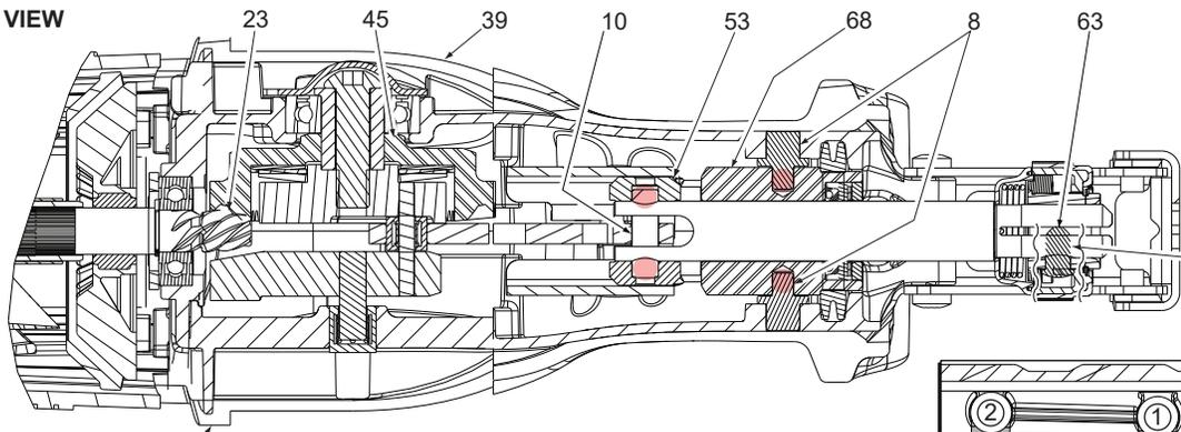
Pin (63) is to be coated with graphite prior to assembly.
