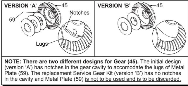
**NOTE:** There are two different designs for Gear (45). The initial design (version 'A') has notches in the gear cavity to accommodate the lugs of Metal Plate (59). The replacement Service Gear Kit (version 'B') has no notches in the cavity and Metal Plate (59) is not to be used and is to be discarded.
