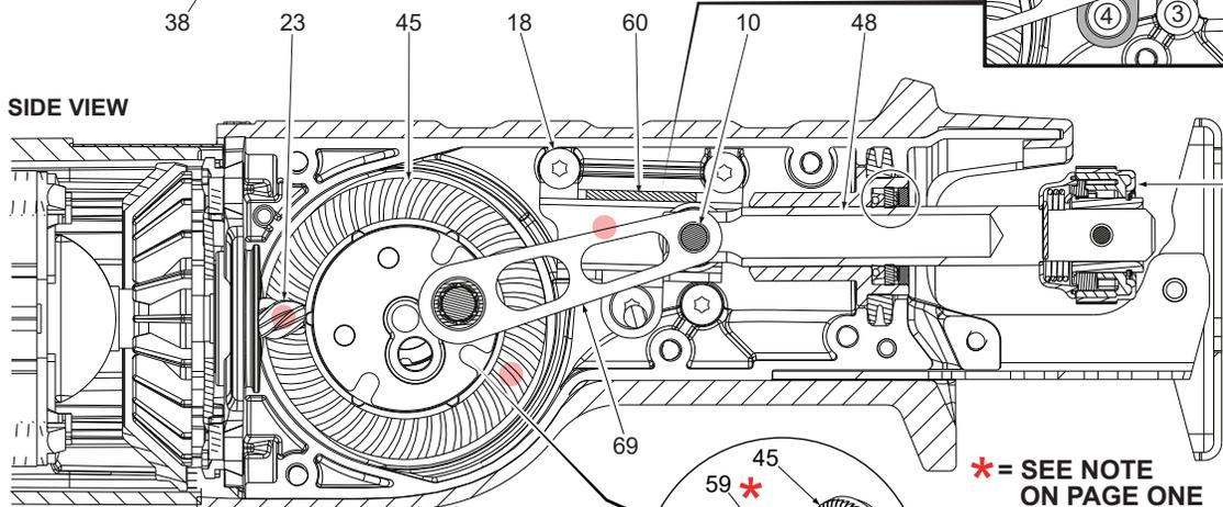
When securing the orbit slot (60), tighten screws (18) in the order shown.
