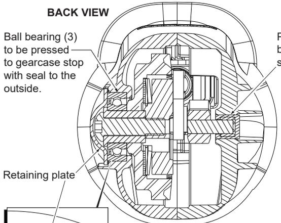
Ball bearing (3) to be pressed to gearcase stop with seal to the outside.
