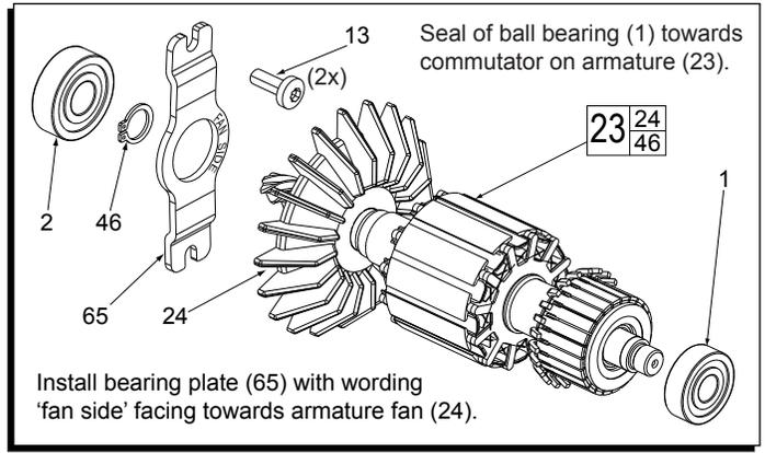
Seal of ball bearing (1) towards commutator on armature (23).
