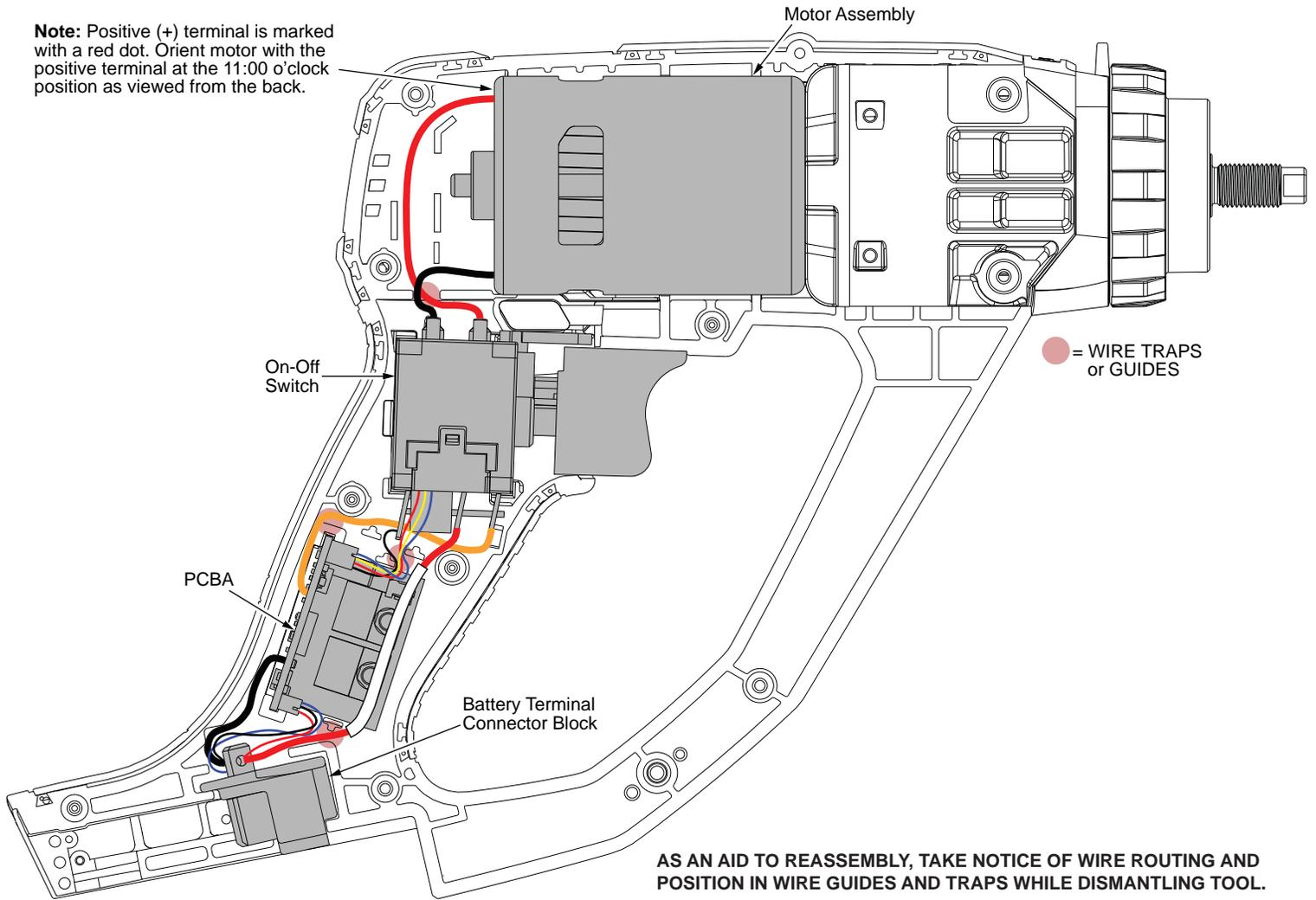
**AS AN AID TO REASSEMBLY, TAKE NOTICE OF WIRE ROUTING AND POSITION IN WIRE GUIDES AND TRAPS WHILE DISMANTLING TOOL.**
