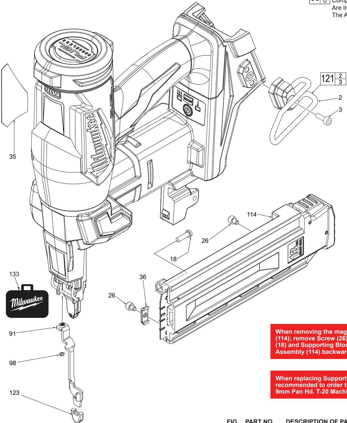
When removing the magazine assembly (114); remove Screw (26), Hex Socket Screw (18) and Supporting Block (36). Pull Magazine Assembly (114) backwards and then twist.
