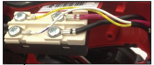
Tuck all switch wires down under the housing tab.
