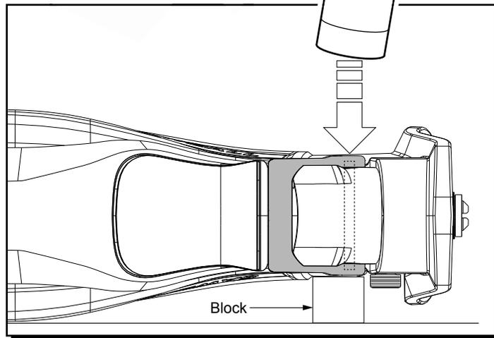
**To properly install the Shoe Release Lever #22 onto the Shoe Pin #23 do the following:**
