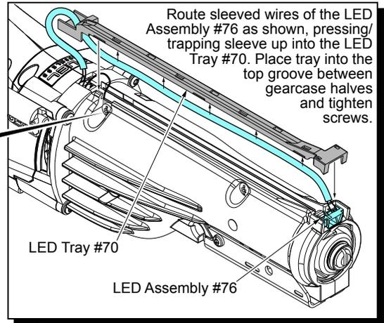
Route sleeved wires of the LED Assembly #76 as shown, pressing/trapping sleeve up into the LED Tray #70. Place tray into the top groove between gearcase halves and tighten screws.
