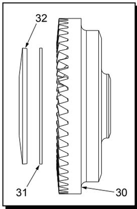
Concave side of disc spring (32) must face toward metal plate (31) and bevel gear (30).
