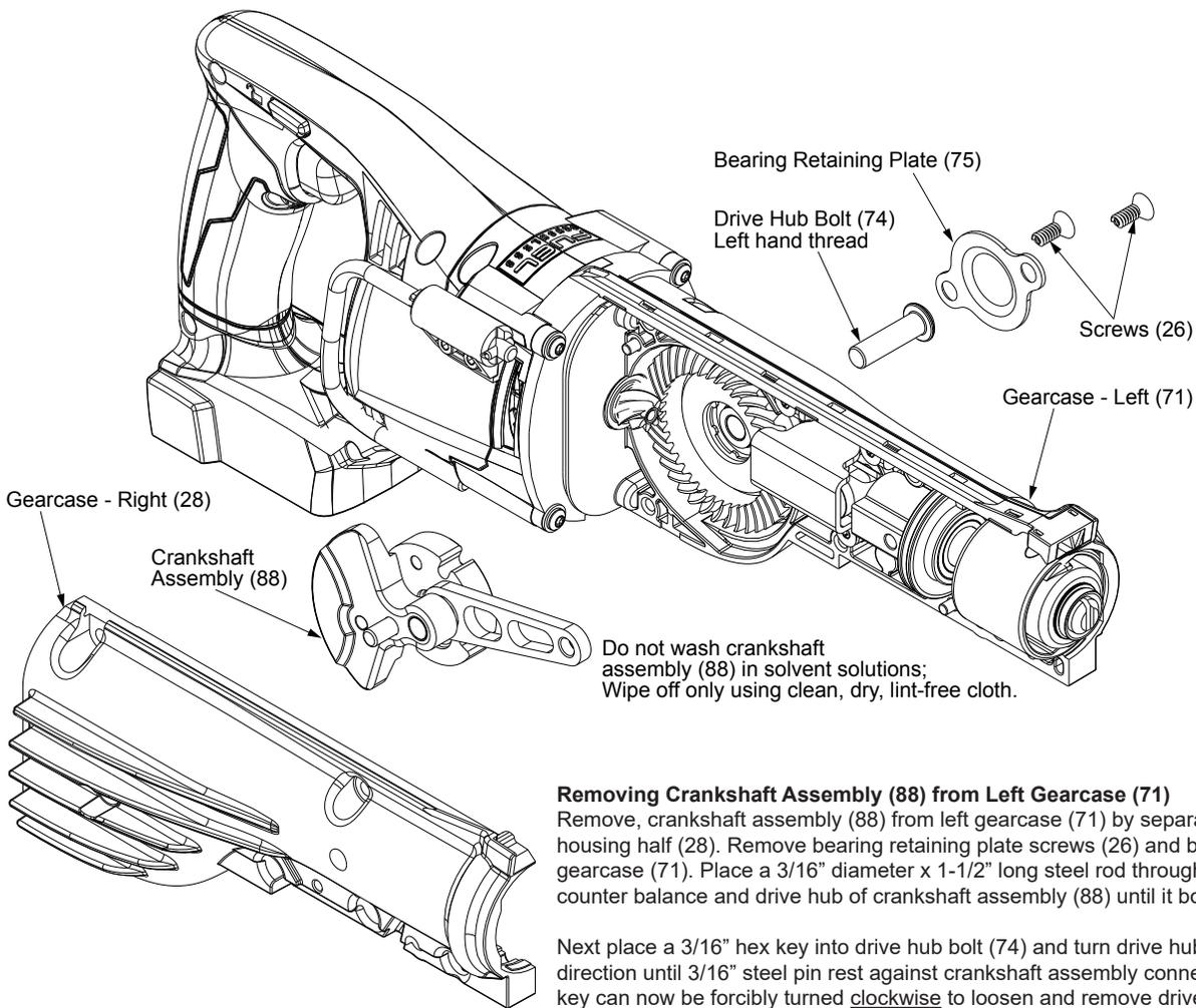
**Removing Crankshaft Assembly (88) from Left Gearcase (71)**
