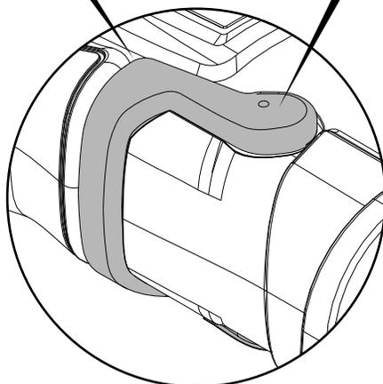
Place the tool on its side on a hard flat surface. Place a small wood block approximately 1-1/8" thick under the tool, between the hard surface and the shoe release lever, directly beneath the pin.
