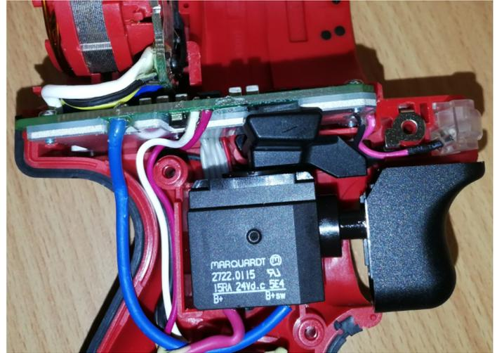
**STEP 8:** Route the PCBA wires connected with battery terminal into the wire channel of left housing as shown.
