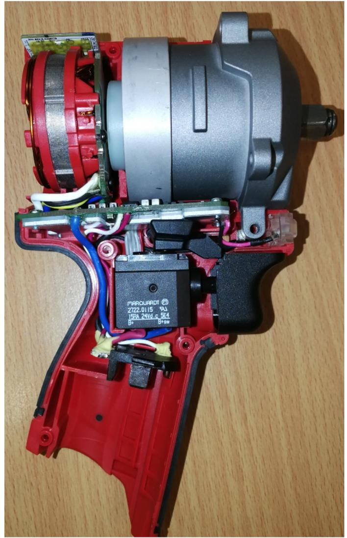
**STEP 11:** Assemble the gear case assembly onto the left housing half and secure with two gear case screws.
