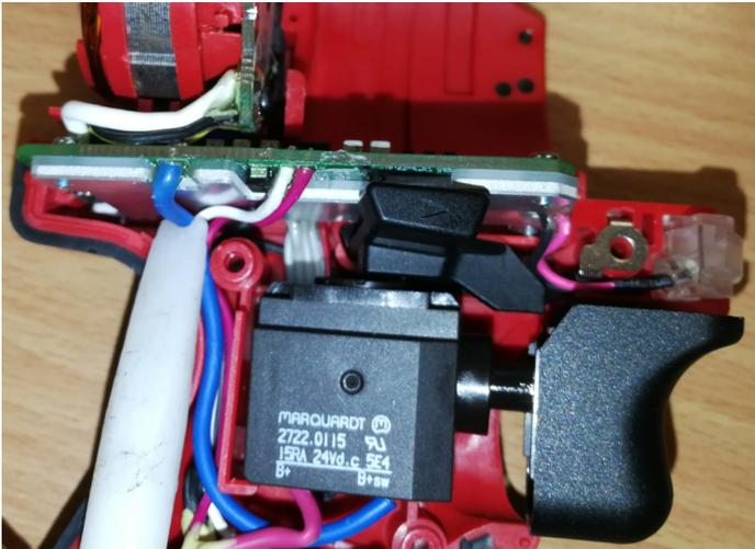
**STEP 9:** Use a plastic/nylon instrument to carefully press blue wire into housing cavity, over the battery terminal wires.
