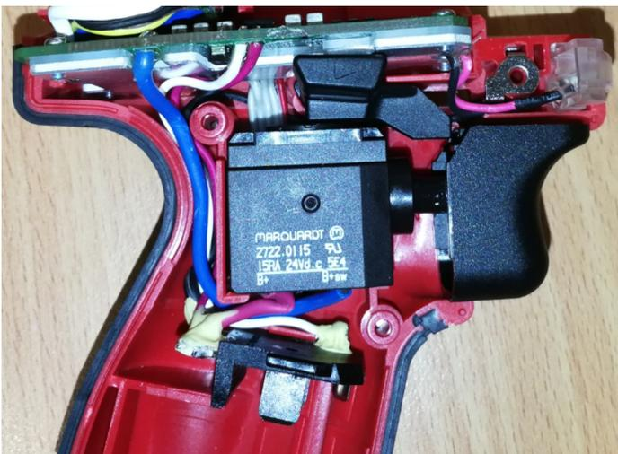
**STEP 10:** Install battery terminal block into the housing half being sure that it is firmly and squarely seated in the cavity.
