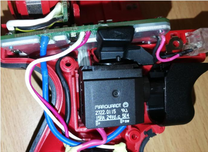
**STEP 7:** Install forward/reverse shuttle and on-off switch into left housing half-support. Be sure shuttle is properly seated over the forward/reverse tab on top of on-off switch.
