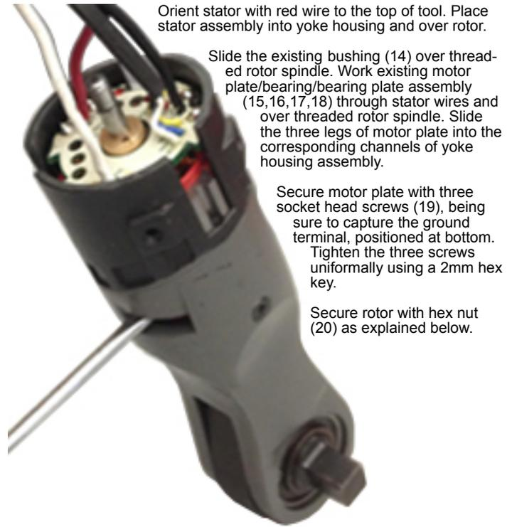
Orient stator with red wire to the top of tool. Place stator assembly into yoke housing and over rotor.
