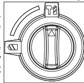
**NOTE:** To engage the hammering mechanism, maintain pressure on the bit. When pressure on the bit is released, the hammering action will stop.
