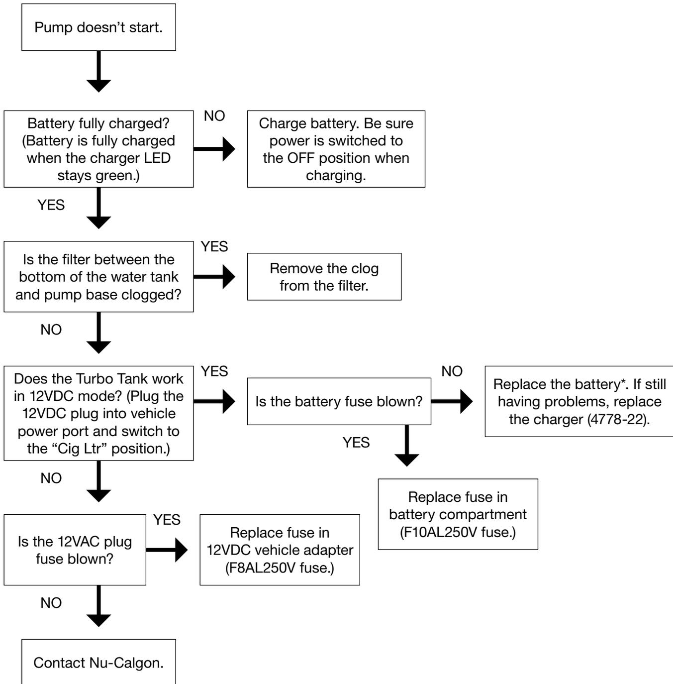
\*Replace with Expert Power EXP 1245, 12VDC 4.5Ah lead/acid rechargeable battery - a product that is readily available in the market.
