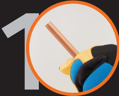
Firmly hold tubing at all times. Keep a safe distance between your hand and the tube's border. Wear eye, face protection and gloves.
