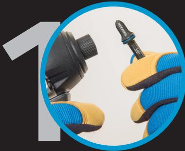
Choose bit size & attach it to the chuck or coupler. Fasten it well. Set the power tool to MAX speed & torque if it is adjustable. Wear eye, face protection, and gloves.
