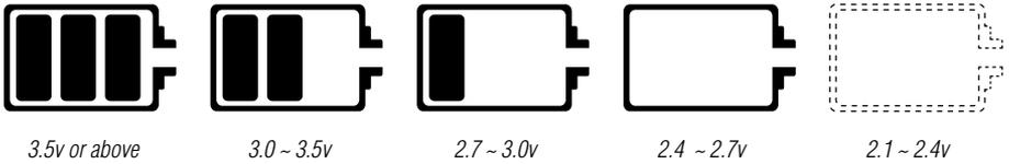
When the battery voltage drops below 2.4 volts, the battery outline will flash and the unit will beep once per minute to alert the low battery condition. When battery voltage falls below 2.1 volts, the shutdown timer is activated. If voltage stays below 2.1 volts for thirty seconds, the DV-22N will beep once and power off.
