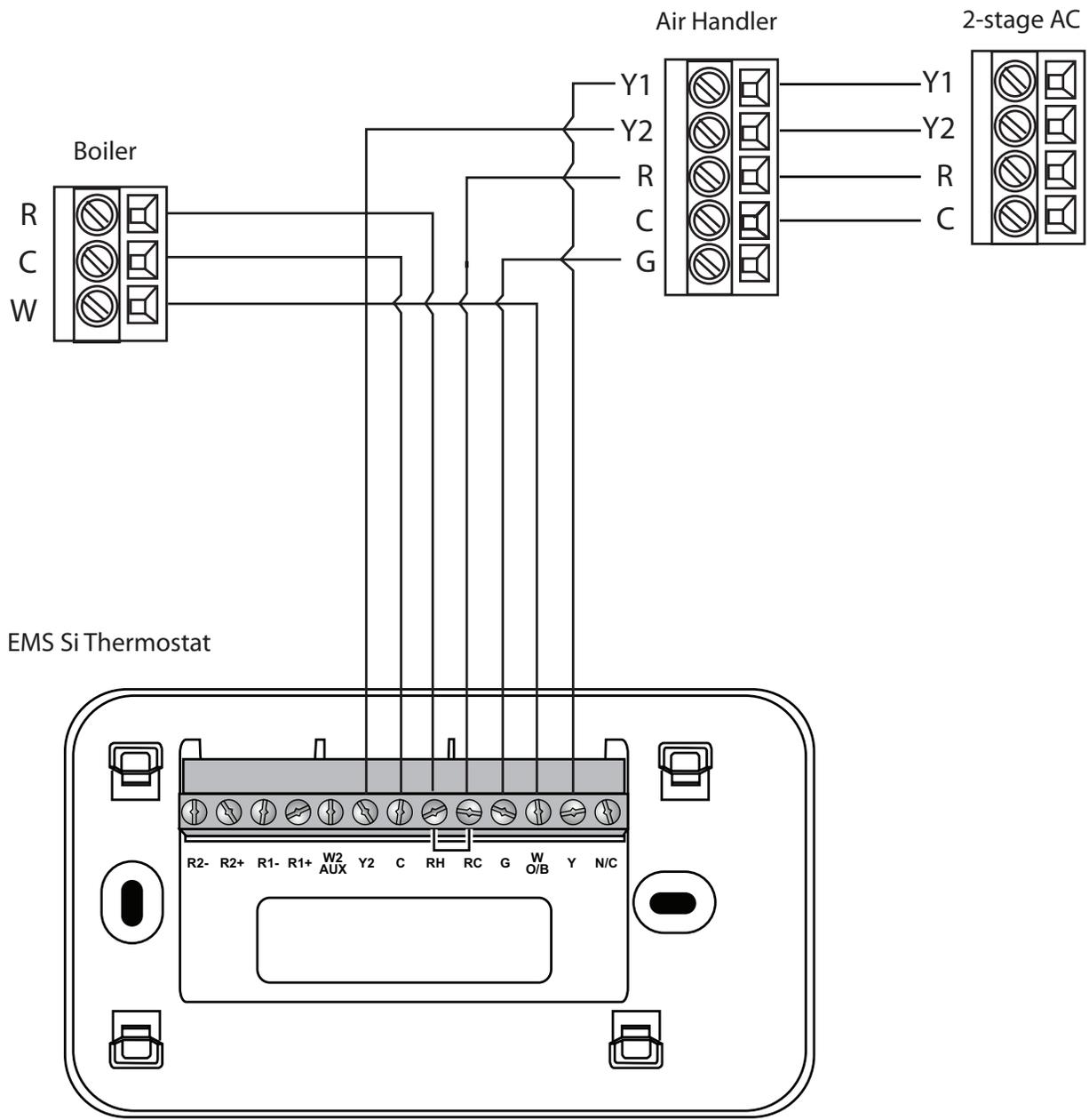
*\* Remove RH/RC factory jumper*
