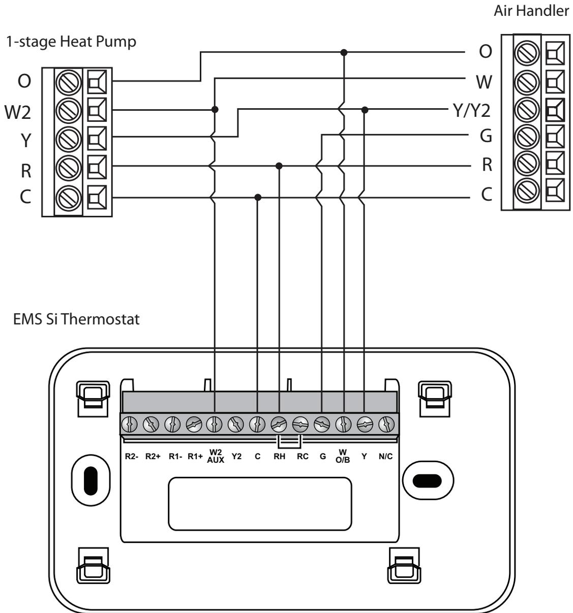
*Single stage heat pump with auxiliary heat*
