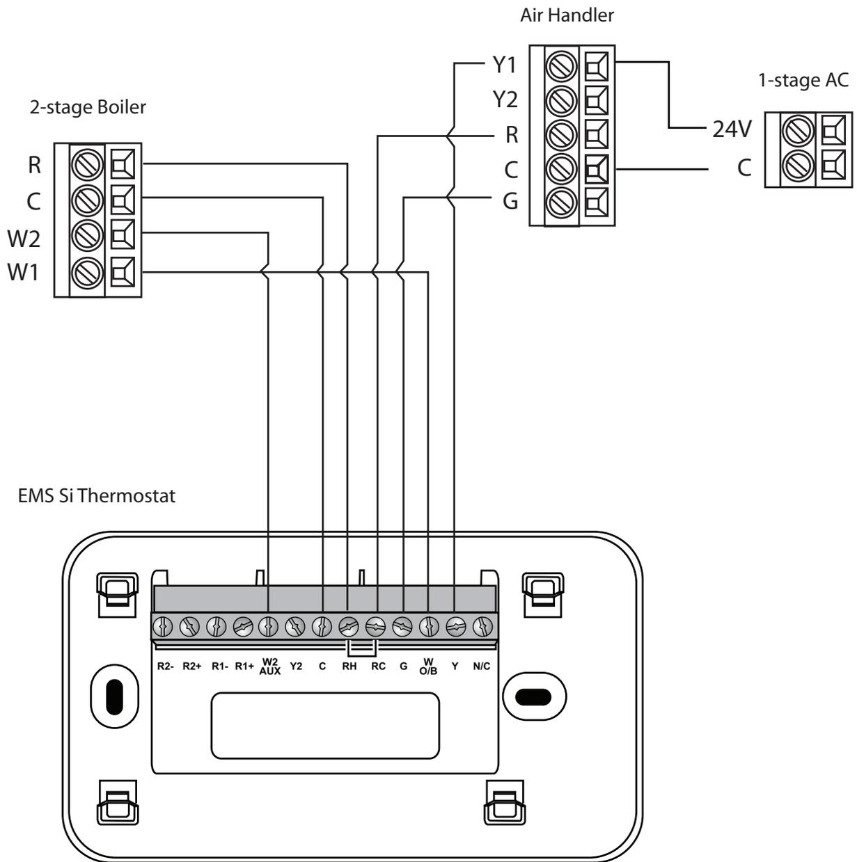
*\* Remove RH/RC factory jumper*
