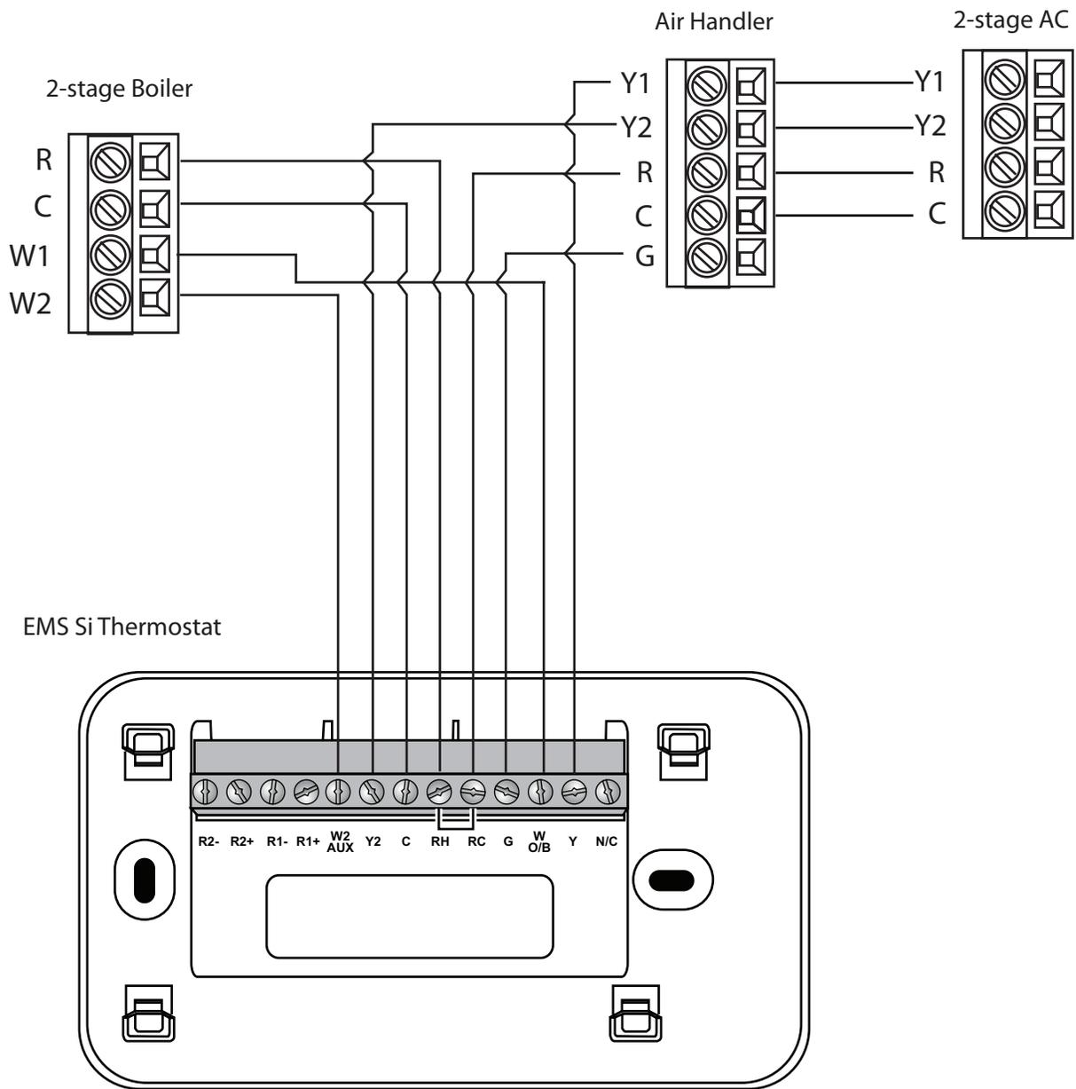
*\* Remove RH/RC factory jumper*
