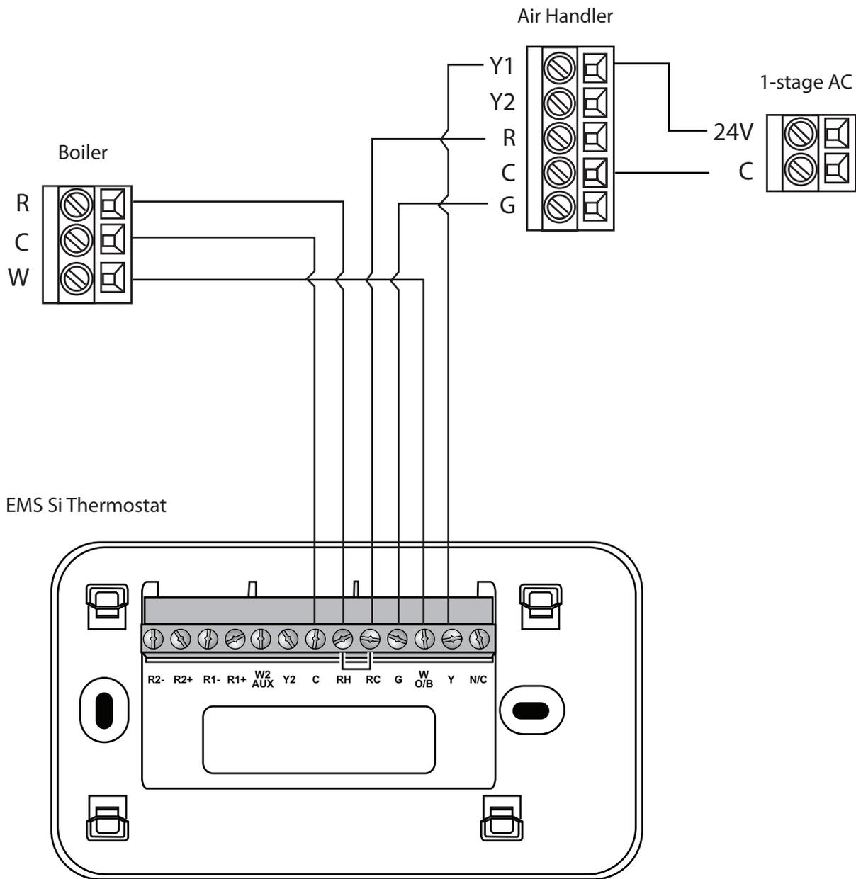
*\* Remove RH/RC factory jumper*
